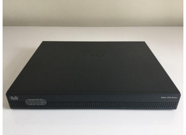
Cisco Router ISR 4321
