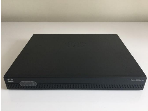
Cisco Router ISR 4321
